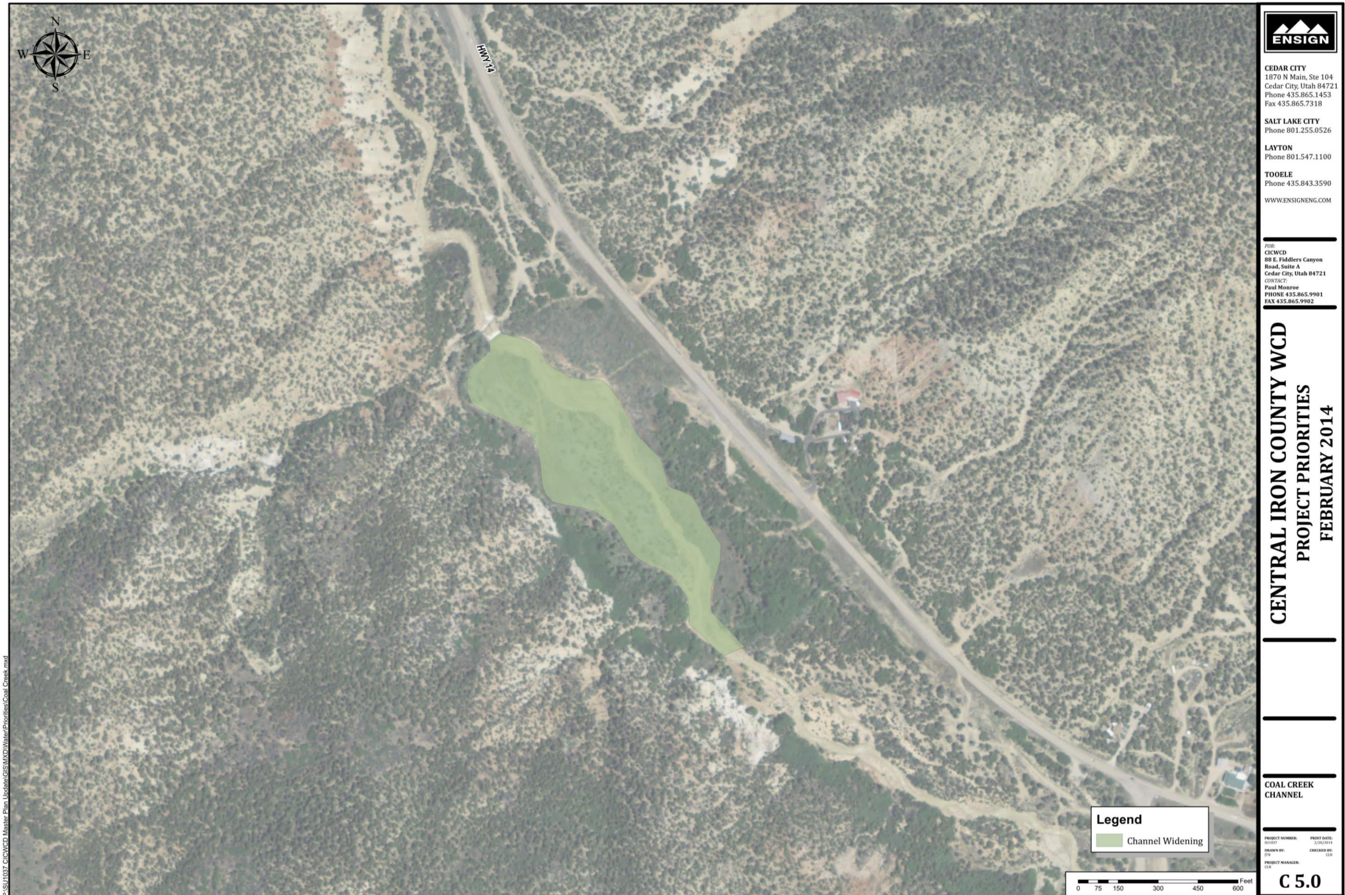
Figure 16 Upper Coal Creek Channel Widening
