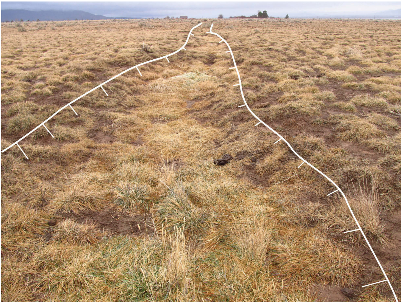
Figure 45. Linear depression 4 to 5 feet wide developed along the Quichapa-southwest fissure (view is to the north). Ticks point toward depression. Photo taken in December 2012.
